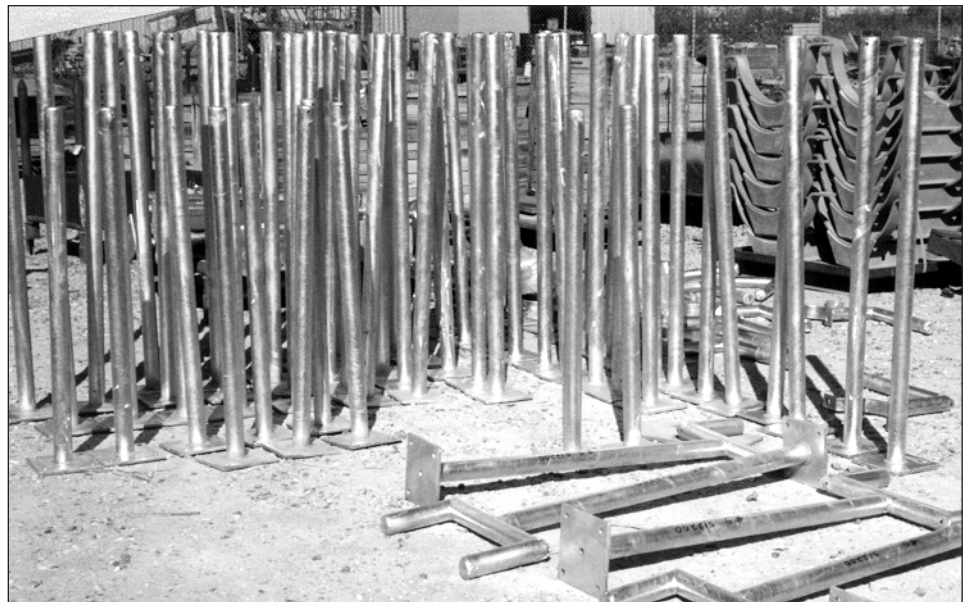
INSTRUMENT SUPPORTS READY FOR FINAL INSPECTION
