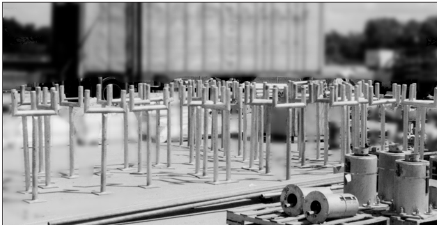
WELDED INSTRUMENT SUPPORTS READY FOR SHIPMENT
